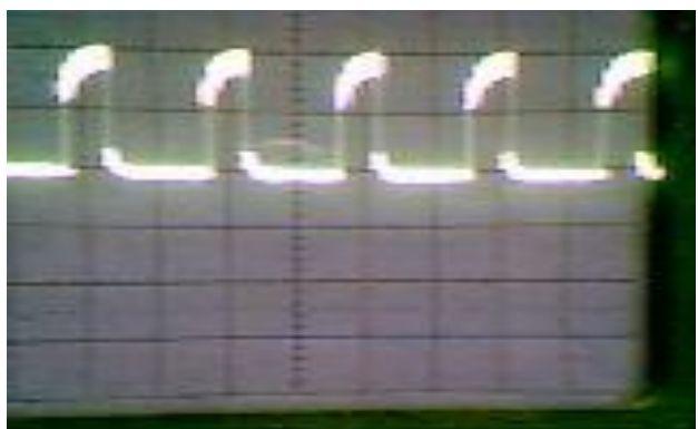
Fig.8. Pulse pattern for a speed of 700 rpm
