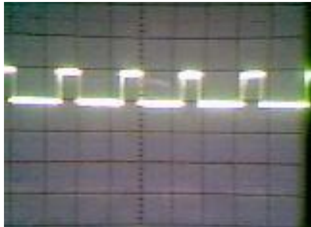
Fig.10. Pulse pattern for a speed of 1200 rpm
